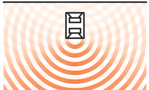
The 8c's directional design avoids early reflections
